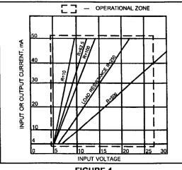
FIGURE 1 INPUT/OUTPUT AND LOAD CAPABILITIES
