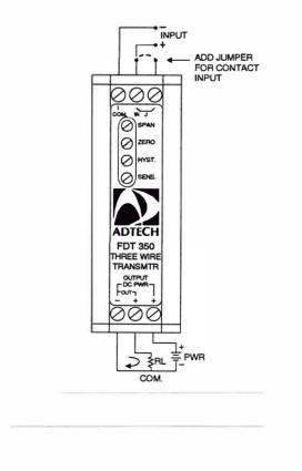
NOTE: For contact input install jumper from terminals 2 to 3.
